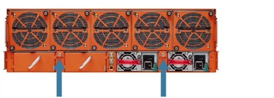
Figure 10 Fan Tray Screw Location on GigaVUE-HC3 Rear
